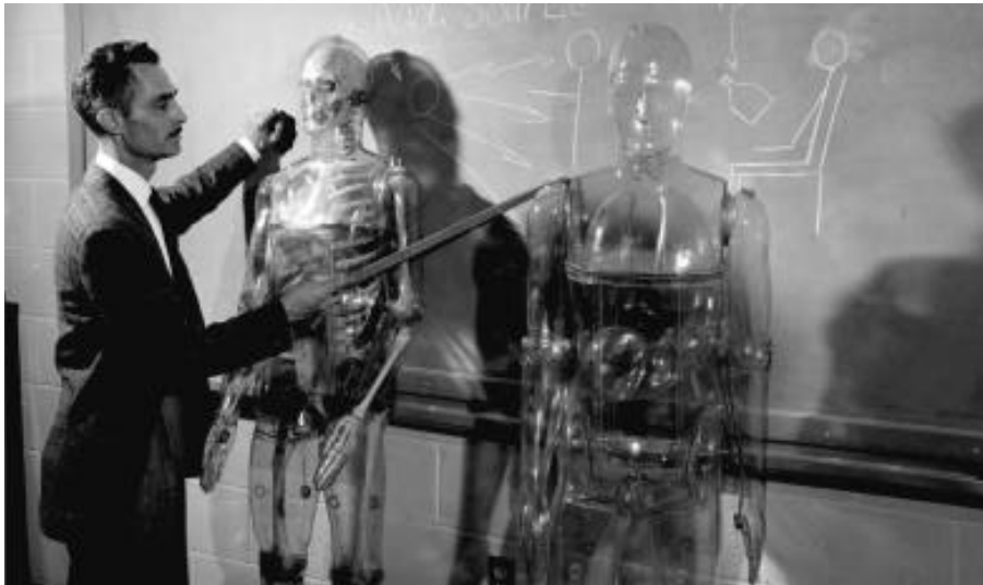
Figure 6. A Captive Audience Wright Langham lectures on the uses of Remab (left) and Remcal in the calibration of the whole-body counters, HUMCO I and II. These plastic “phantoms” enabled the researchers to perform “human” experiments to determine the efficiency of the detectors.
